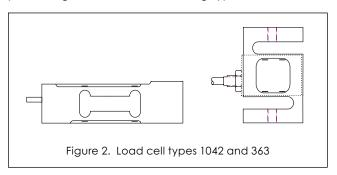
Bending as a measuring principle offers excellent linearity. Bending beams have relatively high strain levels with greater deflection compared to other measuring principles. This in turn means that although the cell is subjected to greater static overload, mechanical stops are more feasible. The dynamic overload capabilities are excellent because of the typical high deflection.
