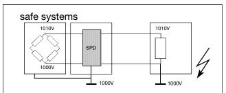
Figure 21. Systems with unavoidable multiple points of earthing should use an SPD to divert surges to a local ground. By doing so, the whole system will rise and fall at the same potential.
