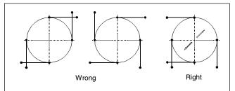
Figure 13. Placing rods as indicated in the left drawings will cause high stresses in the stay rods or rotation of the vessel
