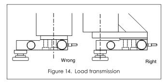
S-type load cells should be mounted in such a way that side forces are reduced to a minimum; they should never be mounted rigidly (even only at one side) between the structure and hopper. The load cell must be orientated in such a way that the cable entry does not affect weighing accuracy.
