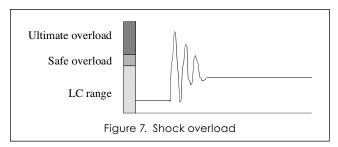
Shock overload can be defined as a sudden change in weight, within a very short period of time, over and above the rated capacity of the load cell. This situation specifically occurs when a relatively small non-elastic item is dropped from a considerable height on the scale. Systems can be protected by incorporating shock insulation pads, or by selecting load cells with a higher rated capacity. Mechanical stops act to assist the protection against shocks.
