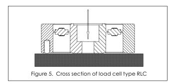
The geometrical design of the sensing element provides enhanced specifications in terms of creep and hysteresis compared to shear and bending as a measuring principle.
