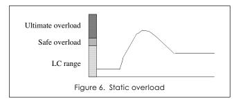
Systems can be protected by incorporating mechanical stops, or by selecting load cells with a higher rated capacity.
