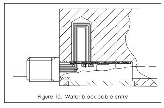
An improvement on the basic cable gland is a water block at the point of cable entry. Here, the main cable terminates at for example a small circuit board with on-going wires leading to the gage area. The block is fully potted to prevent moisture or other contaminants from reaching the critical areas.
