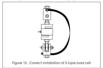
To prevent load cells from being damaged during installation, it is strongly recommended to use dummies or mounting assemblies that can be "locked". Load
